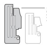
The 72-D3B-2 has a larger needle plate and additional feed dogs.
