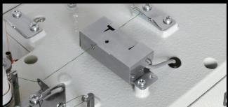
Thread breakage detector SC1761-001
