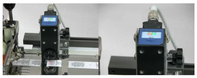
If you did it correctly, when you make sensor light indicate cutting line, the "out" lamp is on.
