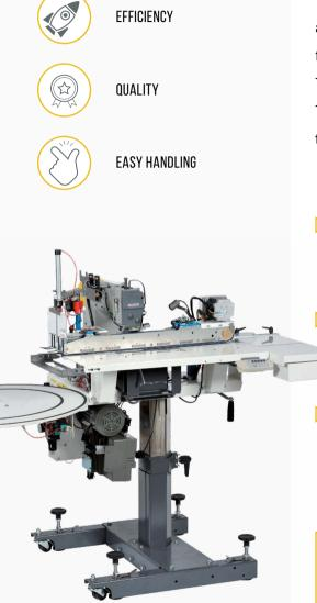
The automatic pocket hemming unit V701, 2 needle lockstitch is a flexible unit with a high level of efficiency and quality output. One unit can supply more sewing lines, following the concept of modular production and space maximization. The unit can perform an average production of 1500 up to 1800 pockets per hour. The innovative transport system allows the units to perform on many kind of fabric thickness from workwear to denim and stretch materials.
